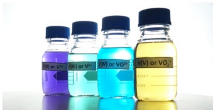
Electrolyte for redox-flow batteries based on vanadium in different oxidation states
